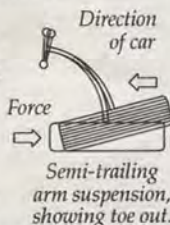
Mazda's exclusive Twin Link design counteracts toe out.
